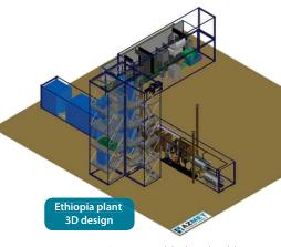
contractors. It is assembled and cold commissioned prior to shipment. Thus, time to install and hot commission on site is limited with minimal changes. Design of supply is flexible and can be adjusted according to the client's needs; with a total supply consisting of six independent modules.
